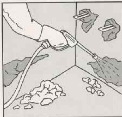
Surface cleaning by chiselling and high pressure water cleansing
